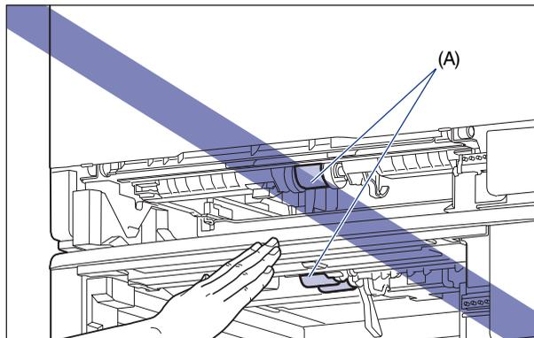
**5** Set the paper cassette in the printer at an angle, and then push it into the printer gently and horizontally.
