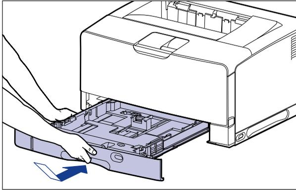
If the paper feeder is installed, set the paper cassette of the paper feeder also.
