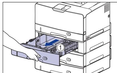
Hold the grips (A) with both hands, raise the front side of the paper cassette slightly ②, and then pull it out completely ③ as shown in the figure.
