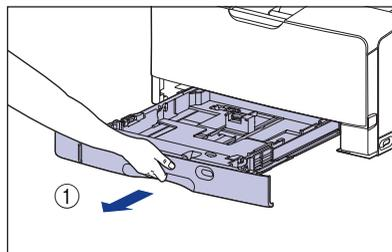
Raise the front side of the paper cassette and remove it from the printer ②.
