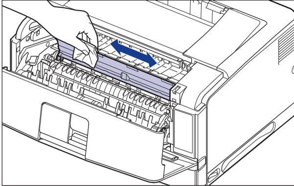
After wiping off the dirt, wipe the area with a soft, dry cloth.
