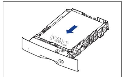
**4** Hold down the paper as shown in the figure, make sure that the paper stack does not exceed the load limit marks (A), and then set it under the hooks (B) on the paper guides.
