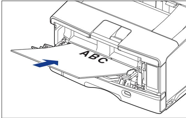
**7** Align the paper guides with both sides of the stack.
