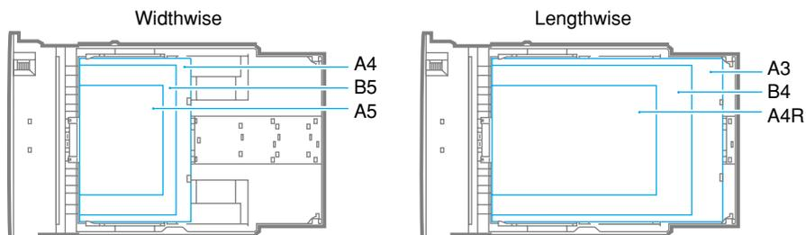
Load A4-size paper widthwise. You can load A4-size paper lengthwise (A4R), but if you do this you must change the [ヨウシノムキ] setting.
